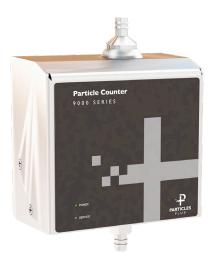
The 9510 Modbus particle counters provide a range of particle size measurement from 0.5 to 25.0  $\mu$ m at a flow rate of 1.0 CFM (28.3 LPM). These sensors allow for efficient particle counting with specifications that exceed the ISO 21501-4 and JIS B9921 calibration standards.
