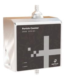
The 2510 and 2510-2 particle counters provide a range of particle size measurement from 0.5 to 25.0  $\mu$ m at a flow rate of 1.0 CFM (28.3 LPM). These sensors allow for efficient particle counting with specifications that exceed the ISO 21501-4 and JIS B9921 calibration standards.
